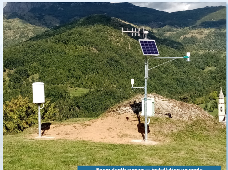
Snow depth sensor — installation example
