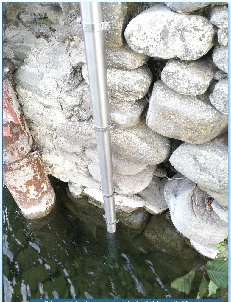
Submersible level sensor — example of installation with stopping pipe
