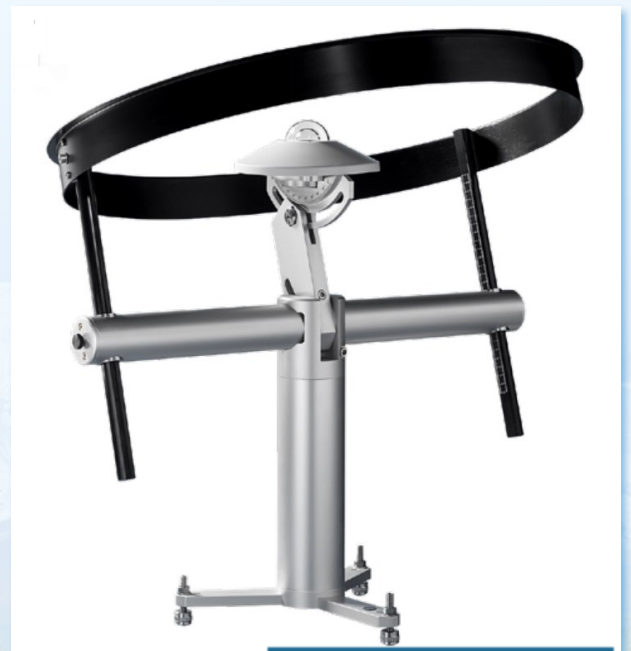
Pyranometer with ring shield
