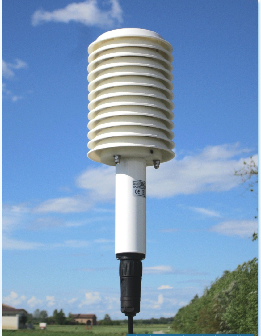
Thermohygrometer with natural ventilation shielding
