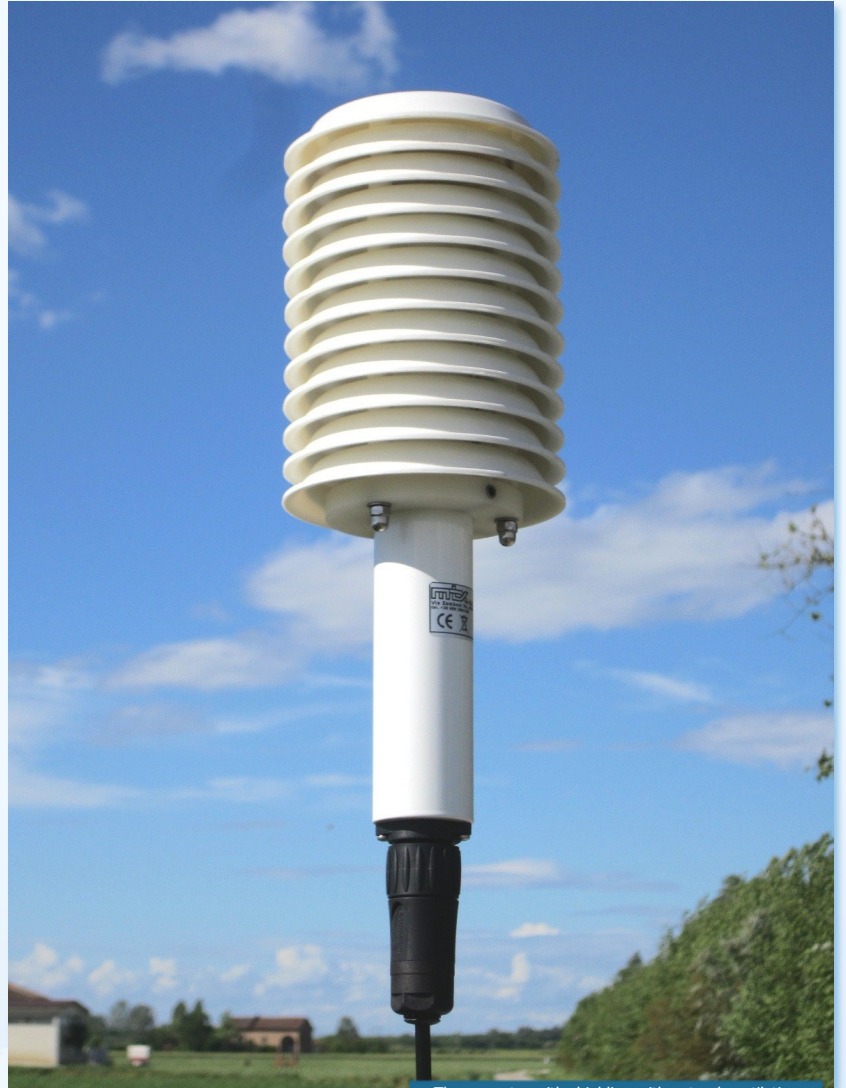
Thermometer with shielding with natural ventilation
