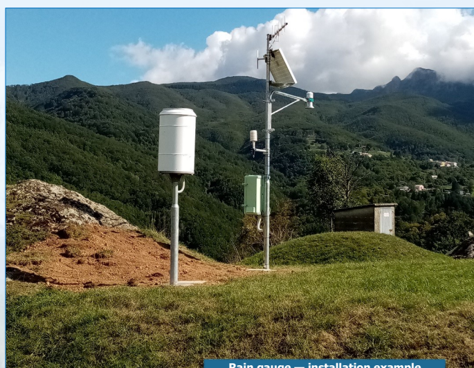
Rain gauge — installation example
