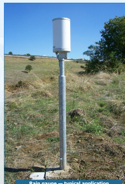
Rain gauge — typical application
